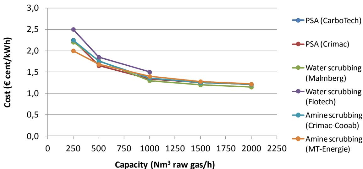
**Figure 12.** Costs for biogas upgrading to biomethane for different upgrading technologies and capacities (Source: (Persson and Wellinger, 2006) ).
