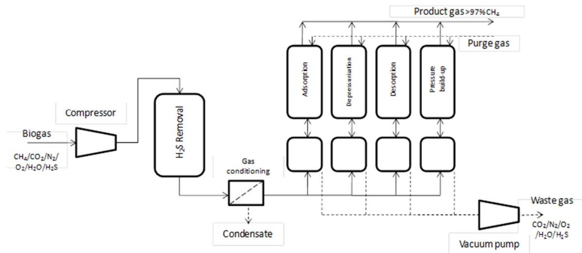
**Figure 7.** Pressure-swing adsorption schematic
