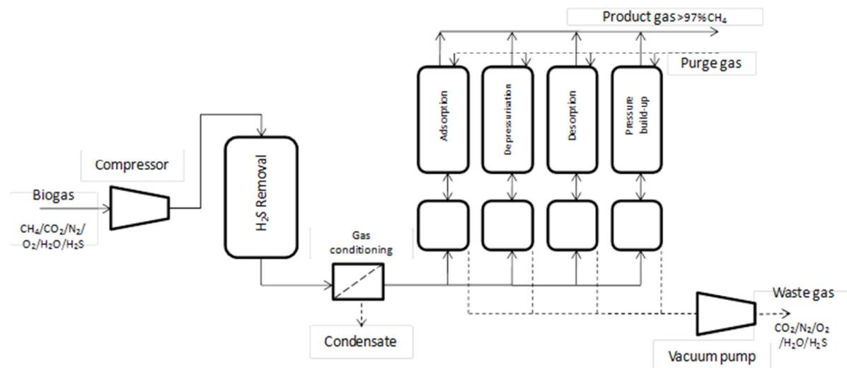
**Figure 7.** Pressure-swing adsorption schematic
