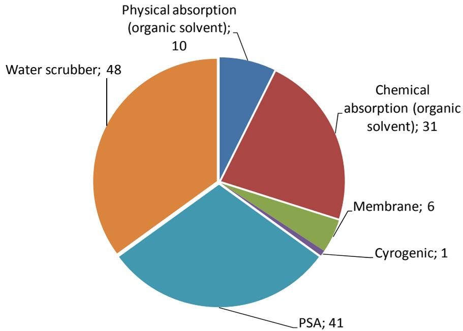
**Figure 4.** Biogas upgrading in Europe – number of biogas upgrading units and technologies (Source: IEA Bioenergy 2011).
