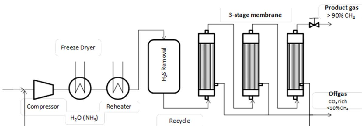
**Figure 10.** Flow sheet for membrane biogas purification process
