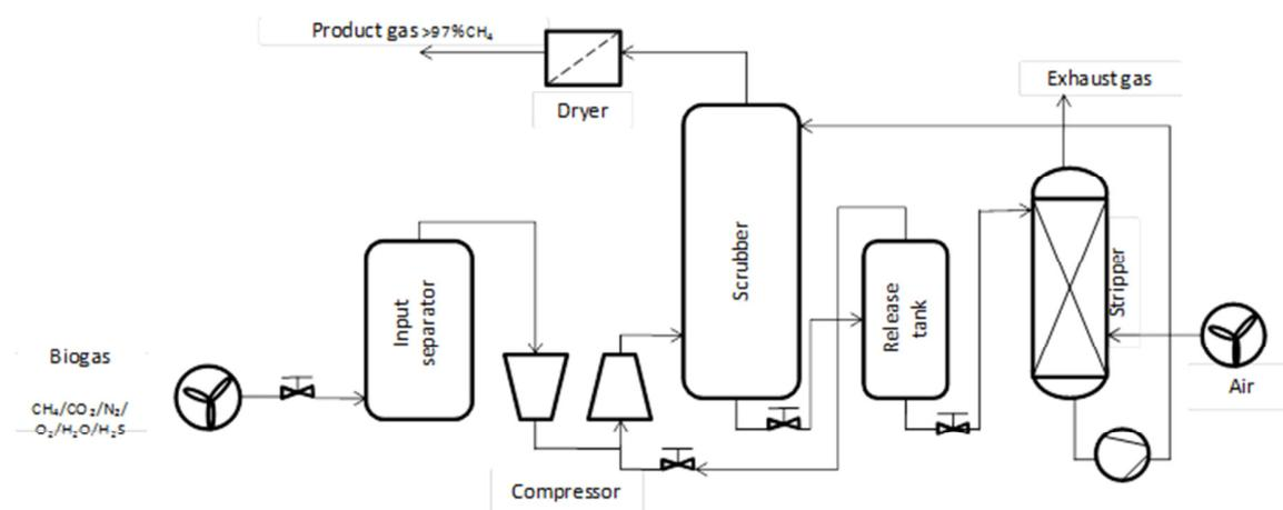
**Figure 8.** Flowsheet for water scrubbing technology (Adapted after ISET, 2008)
