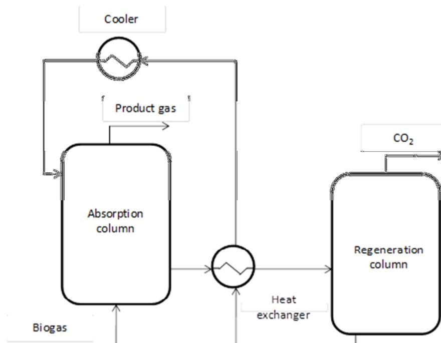
**Figure 9.** Flowsheet for chemical absorption process
