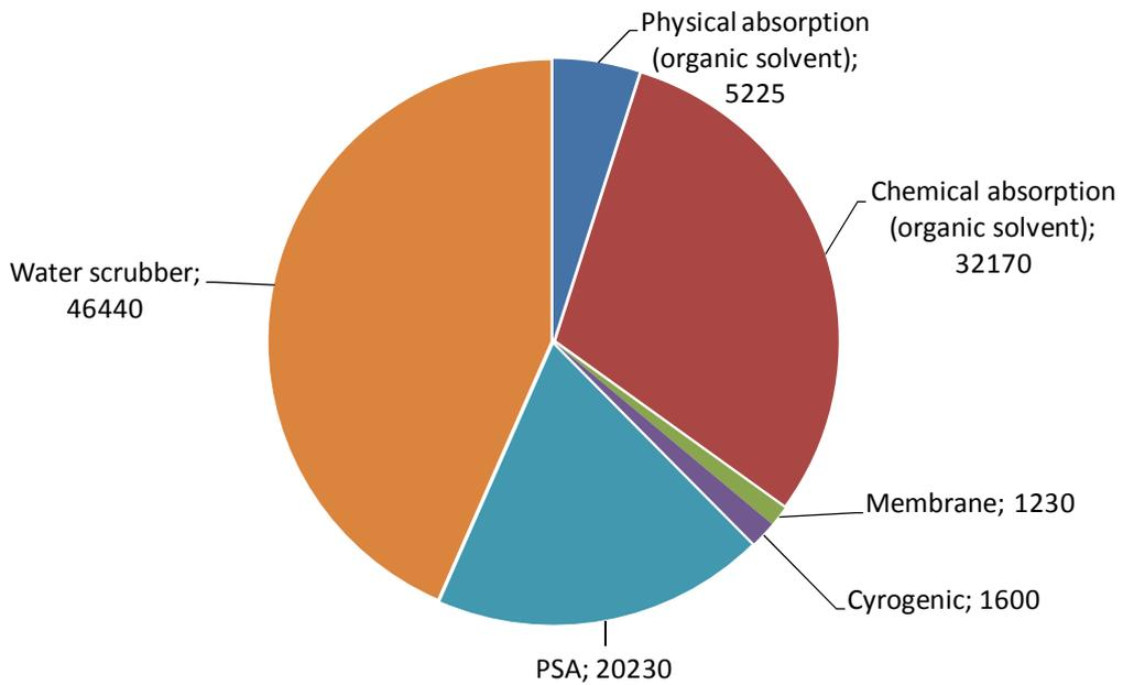
**Figure 5.** Biogas upgrading in Europe – biogas upgrading technologies and capacities (in m<sup>3</sup>) (Source: IEA Bioenergy 2011).
