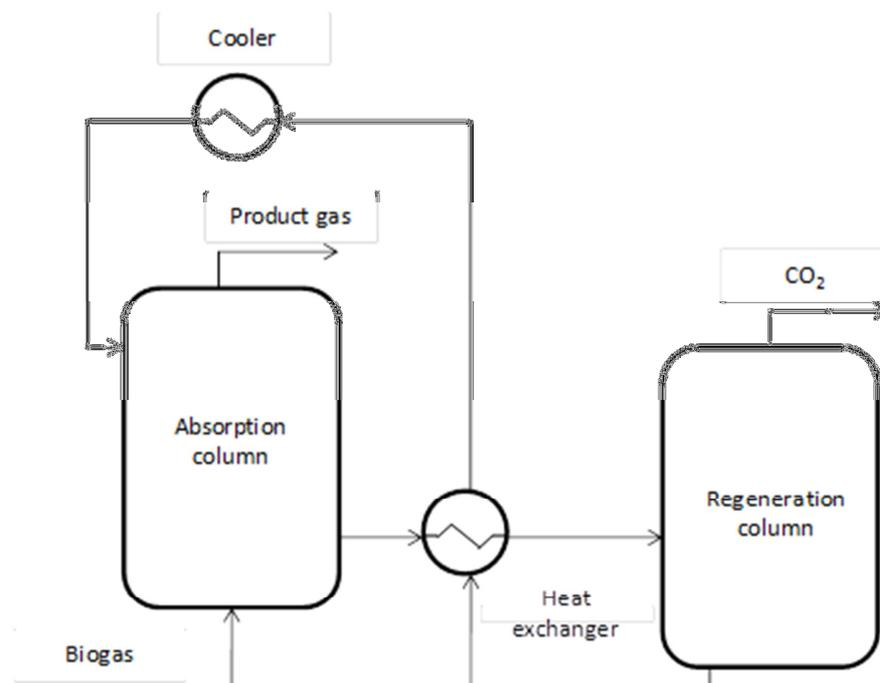
**Figure 9.** Flowsheet for chemical absorption process
