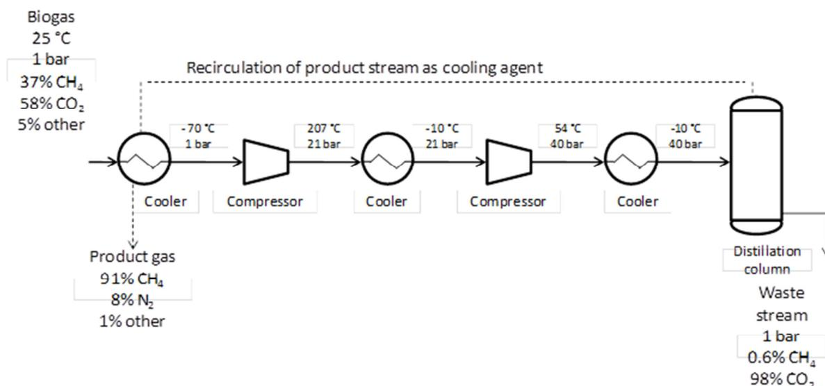
**Figure 11.** Flowsheet for cryogenic biogas purification process (Courtesy: ISET, 2008)
