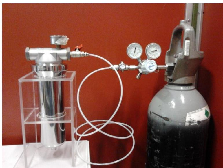
**Figure 3.** CO<sub>2</sub> pressurisation unit with CO<sub>2</sub> bottle.
