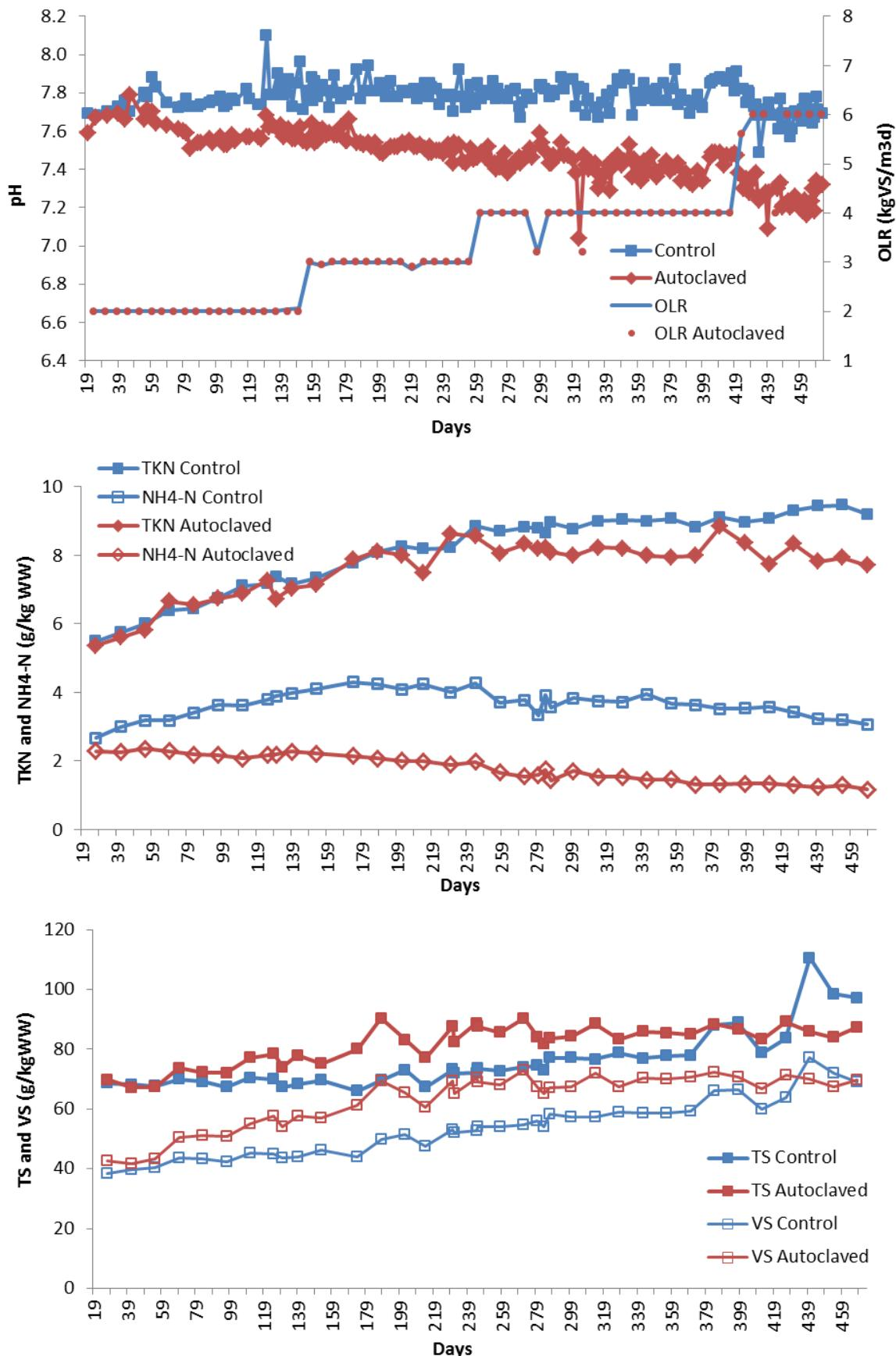
**Figure 6.** Reactor parameters from reactors R1 and R3 during days 19-470.
