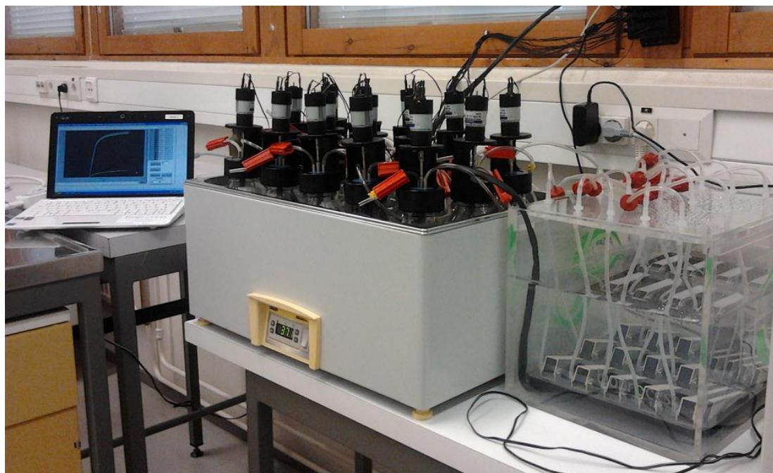
**Figure 4.** Biochemical methane potential testing equipment used in all assays.
