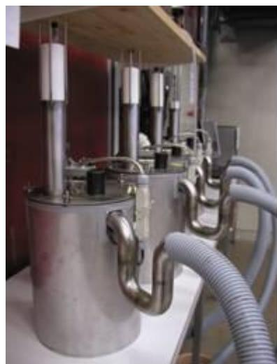
**Figure 2.** CSTR reactors used for treating untreated and autoclaved food waste.
