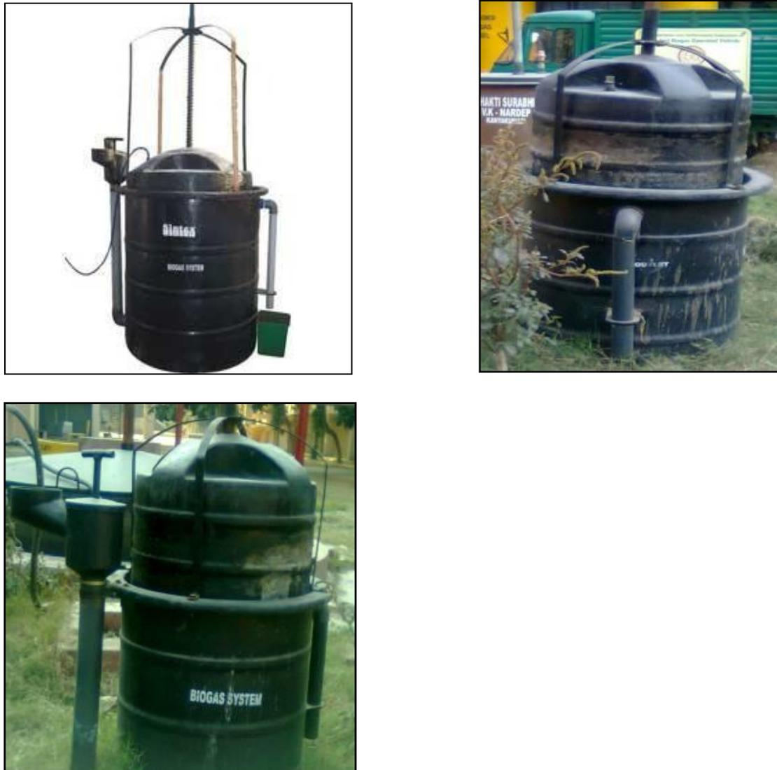
**Figure 10.4** Experimental semi-continuous biogas plant installed in the campus
