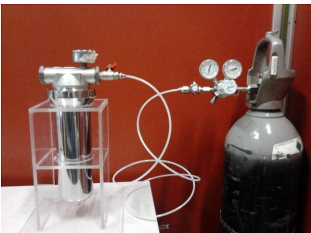
**Figure 1.** Pressurisation unit connected to gas bottle.
