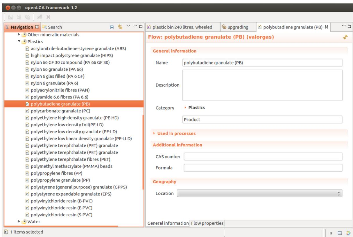
**Figure 8.** Choice of plastic flows in the ELCD version 3 database under openLCA v1.2.9. The outer thread of the plastic wheels on the bin have been represented by 605 g of polybutadiene granulate per wheel.
