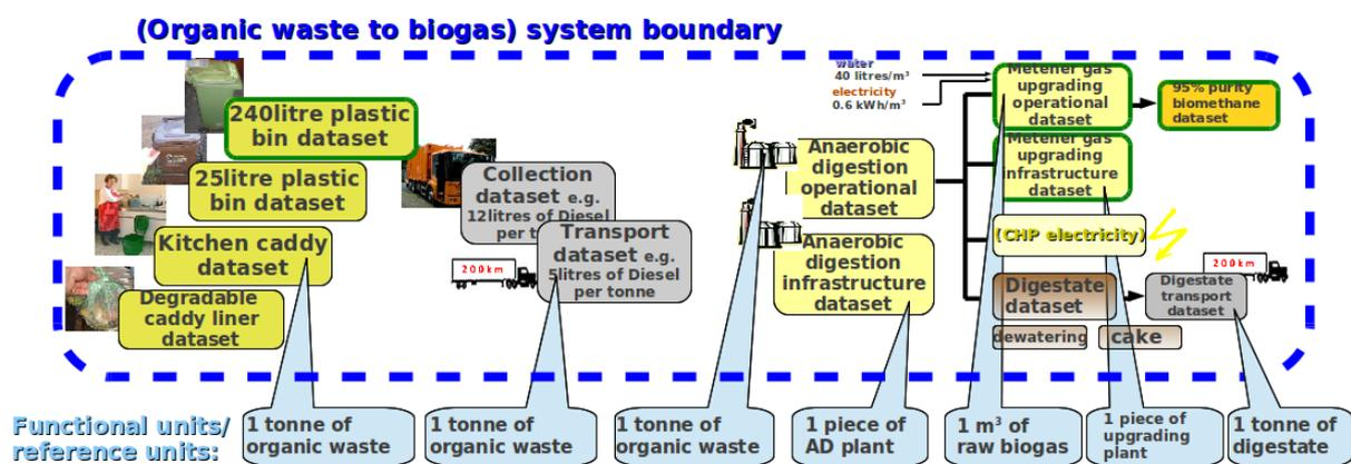
**Figure 3.** Proposed discretisation into datasets of a simple organic waste to biogas process chain. Events or process stages are depicted chronologically from left (collection) to right (digestate residue). Each box represents a potential LCA dataset. Flows in biogas upgrading are given per volume of **upgraded** biogas (not raw biogas).
