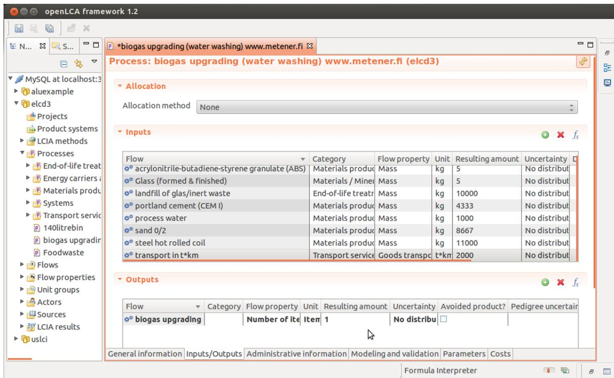
**Figure 5.** Input flows in the biogas upgrading infrastructure process generated in openLCA. There is a single output - one piece of upgrading plant.
