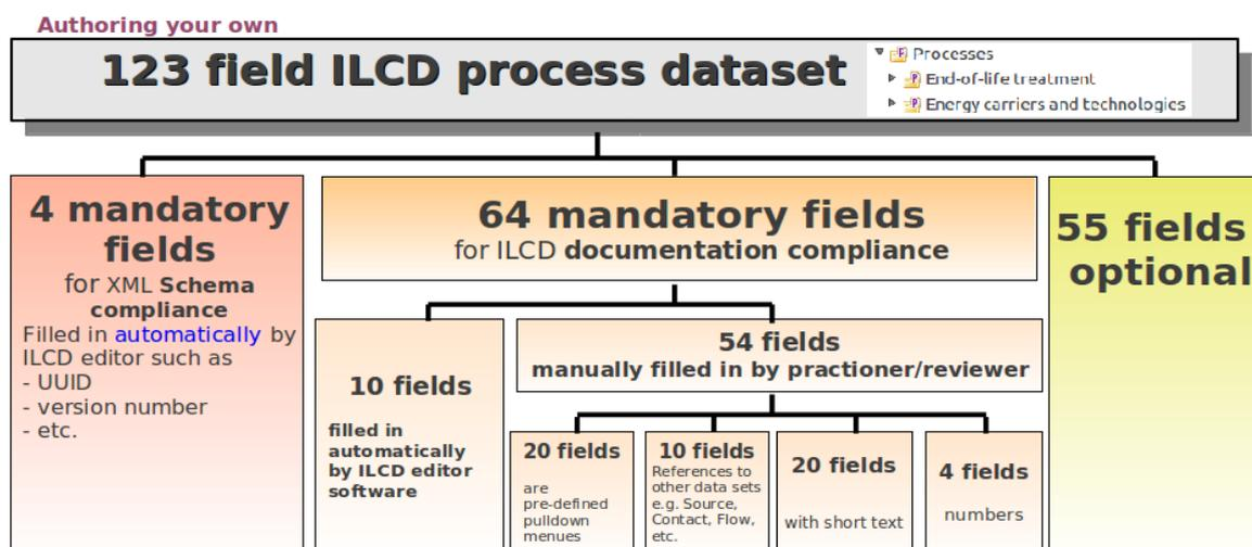
**Figure 2.** ILCD process datasets contain a total of 123 fields that can be populated with data or metadata. Generating ILCD dataset is accomplished with openLCA or the ILCD editor. The ILCD editor stores the data fields in a standardised \*.xml file.
