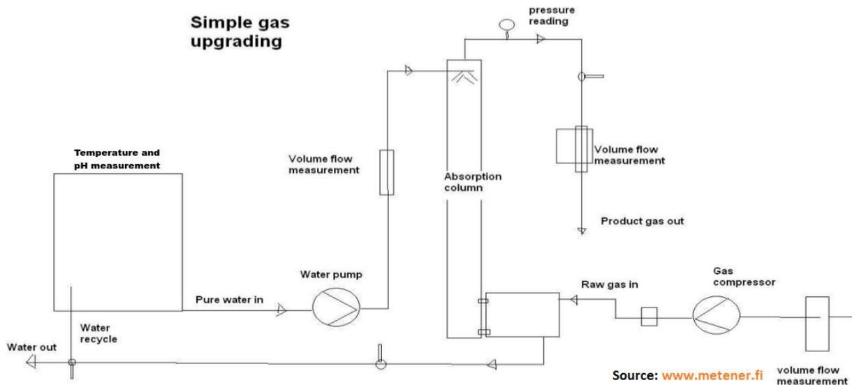
**Figure 4.** Flow diagram of Metener type water scrubbing rig in 2011 involving a water column. Source: <http://www.metener.fi>.
