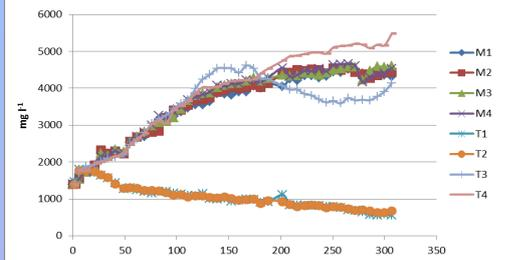
Slow accumulation of VFA in a thermophilic digester fed on food waste
