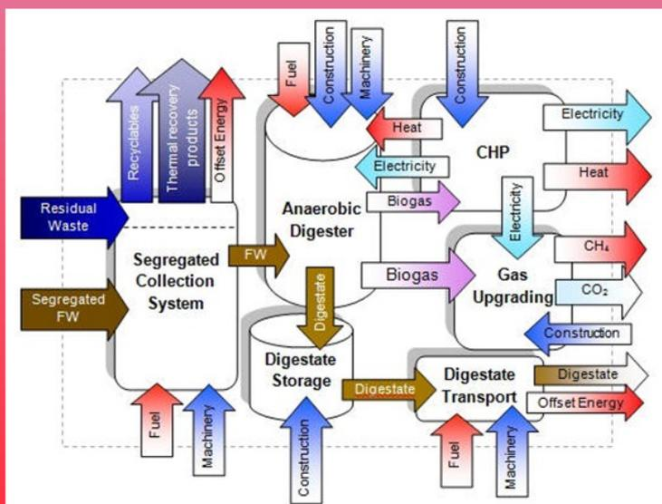
*Energy inputs and outputs in the anaerobic digestion of source segregated food waste*
