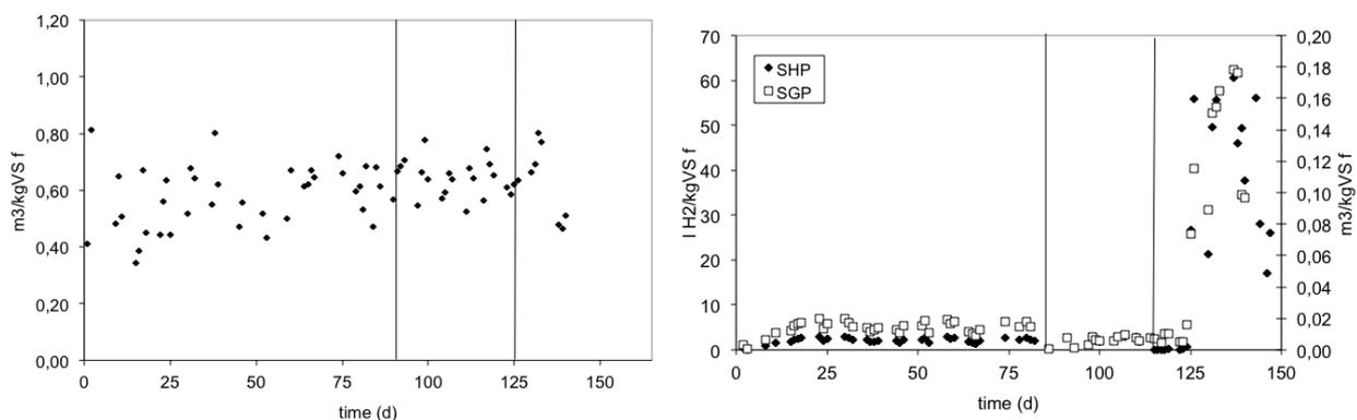
**Figure 2.** Specific gas production and specific hydrogen production in first reactor, and specific gas production in methanogenic reactor during the whole experimental test.
