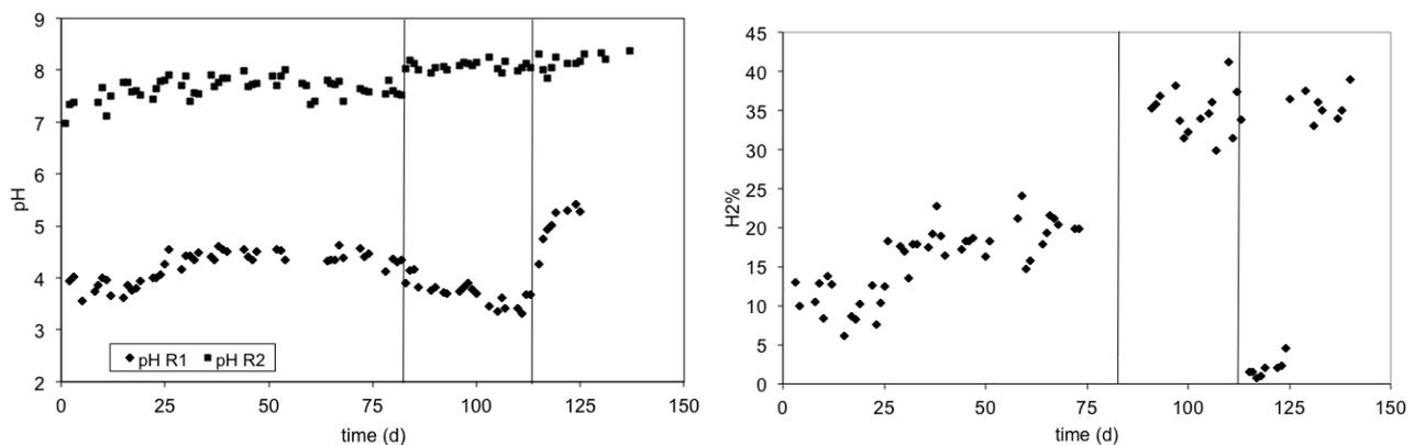
**Figure 1.** pH variation of two reactors and gas composition (H<sub>2</sub> percentage) in the first phase during the three runs.
