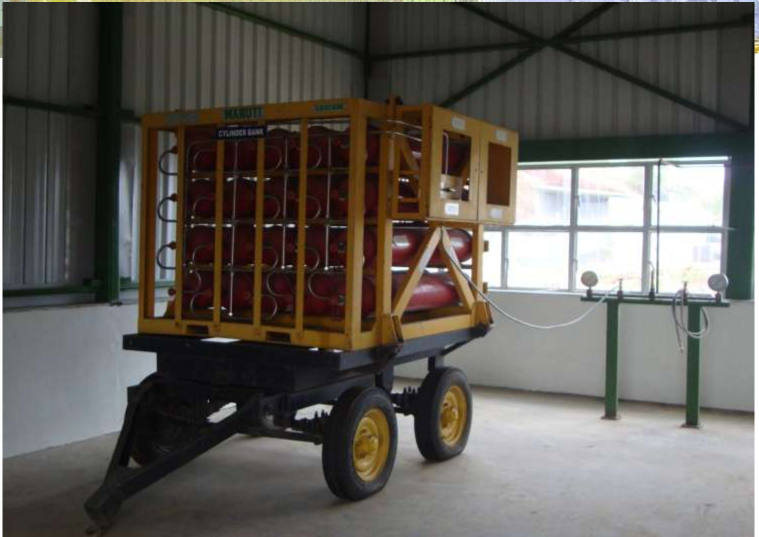
Cascade of 20 cylinders of 80 ltr. Capacity each at Talwade, Nasik
