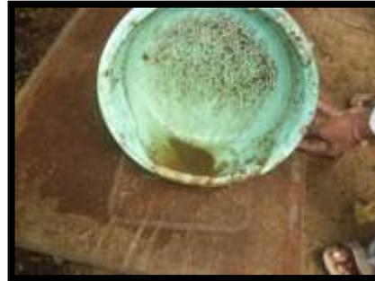
Filtration of slurry by **sieve**
