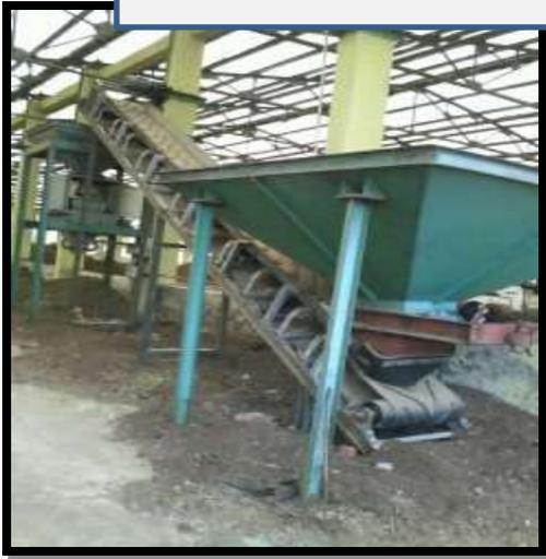
Solid and dried slurry separator
