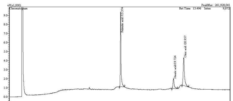
Fig.3 Chromatogram of 50mg/l standard fatty acids solution
