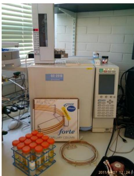
Fig. 2 Samples are ready for analysis, also shown are the GC (Shimadzu 2010) and column used in this study.
