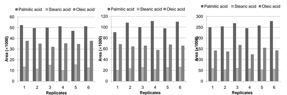
Fig.4 Precision of detector response following the sequential injections LCFAs standards (Concentration from left to right are 50mg/l, 250mg/l and 500mg/l)
