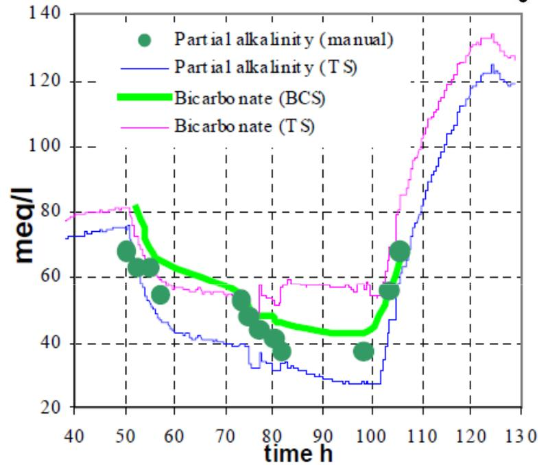
Figure 4: Bicarbonate and partial alkalinity measurement
