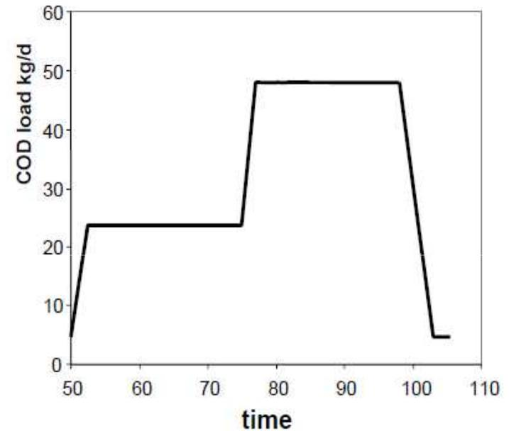
Figure 2: Organic overload to the reactor
