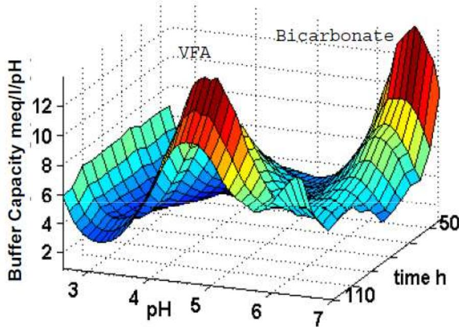
Figure 1: Buffers evolution from bicarbonate alkalinity to VFA during overload
