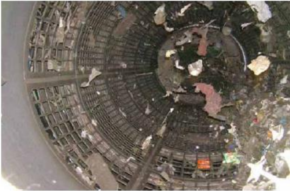
Figure 2: Waste separation using a trommel screen
