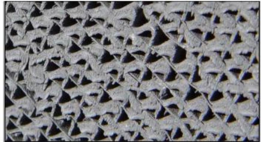
Silicate layers on a catalytic after-burner
