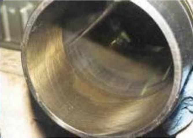
Gold-coloured siloxane layer on the inner surfaces of a cylinder
