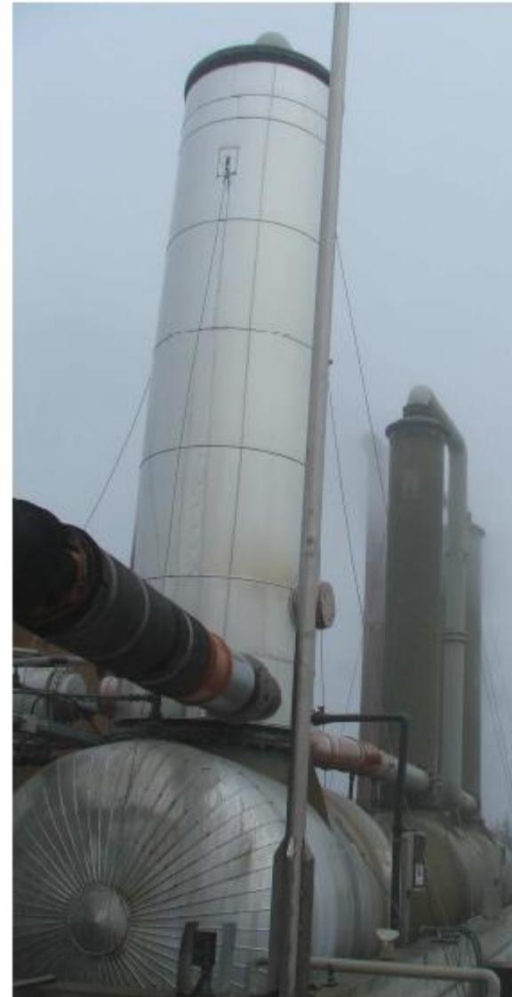
ammonia is stripped out from the digestate using the counter-current exhaust air from the CHP unit (some 80-90° C) and then recovering ammonium sulfate in the second step of the process.
