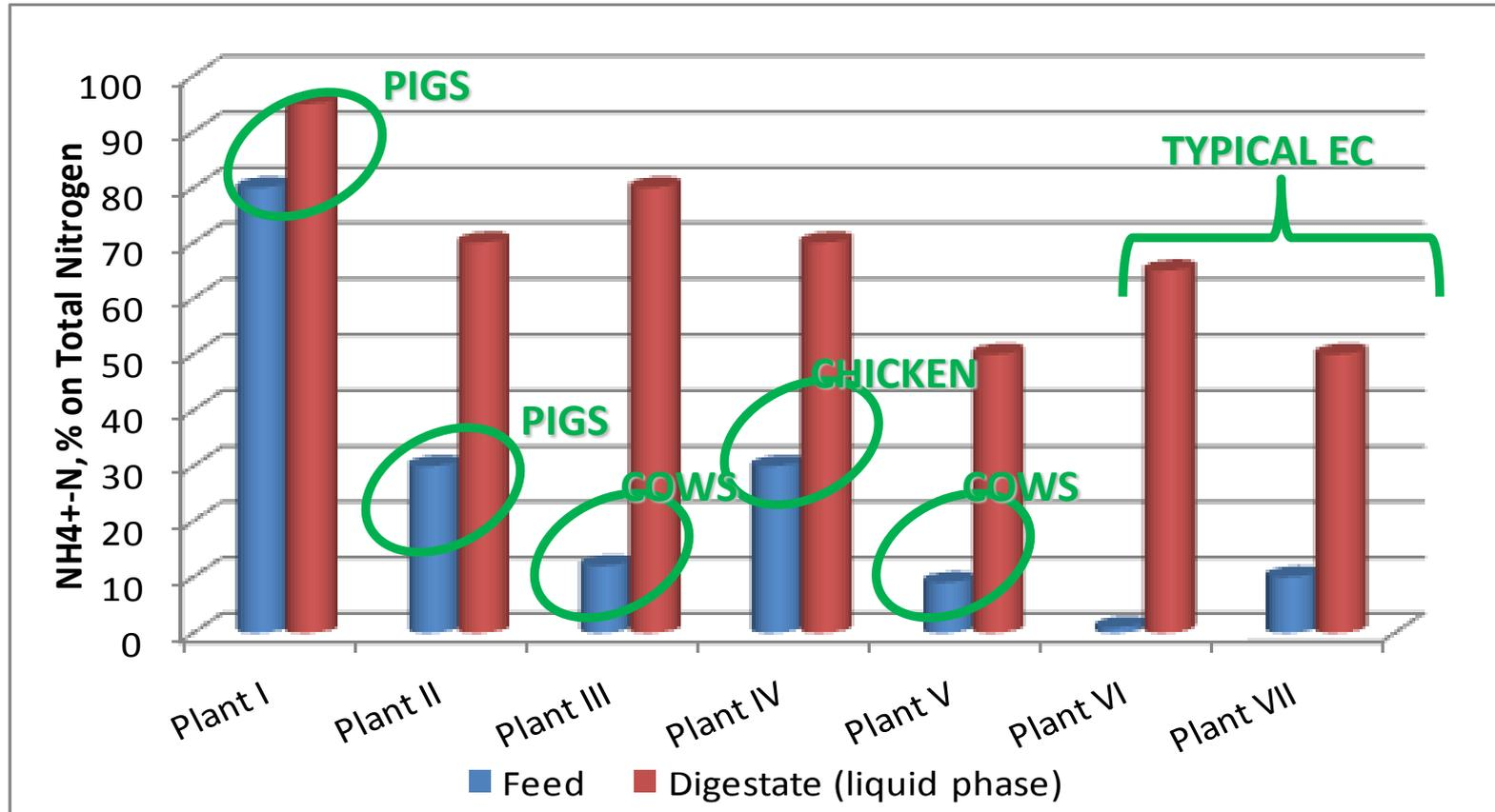
Typical nitrogen distribution in influent and effluent of Italian anaerobic digesters treating livestock effluents, energy crops and agro-waste
