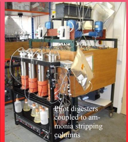
Pilot digesters coupled to ammonia stripping columns
